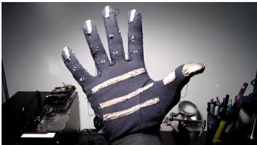
Figure 1: The Keyglove - a wearable, wireless, open-source input device
