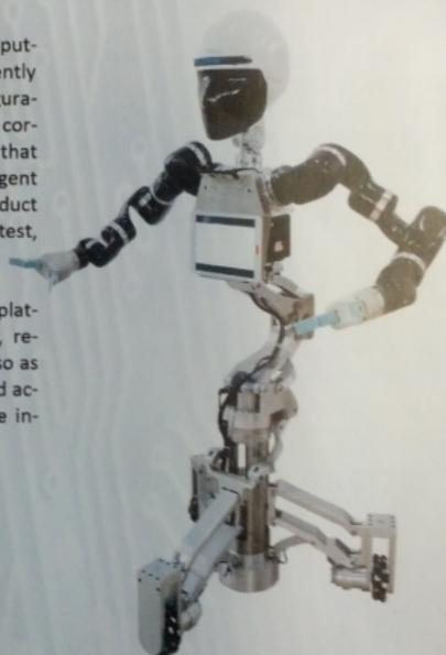
AUBO harmonic-drive actuators, ca. 1500 USD apiece, spindle driven torso lift, ca. 1.40..1.80 m, 3x NUCs on board
