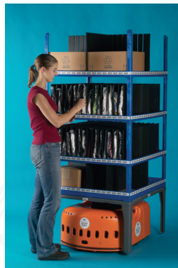
Example of a Kiva Systems Rack, Driver, and Picker [WDM07]
