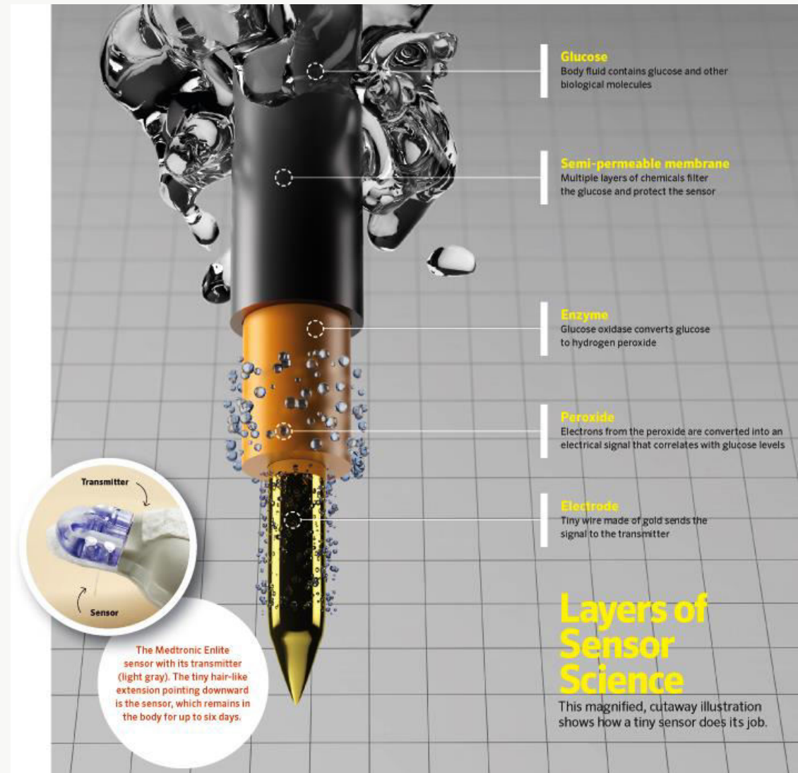
Figure 8: CGM Sensor Components [7]
