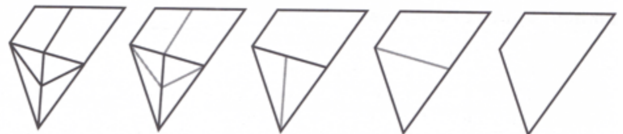
FIGURE 4.3.2 Merging polygons into a single convex polygon.
