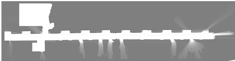
Figure: Grid-map created with Player/Stage on a Pioneer 3-AT with a Hokuyo UTM-30LX laser ranger (~60 meters) attached
