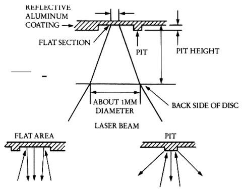
Figure 4. Relation between pits and photodetector output.
