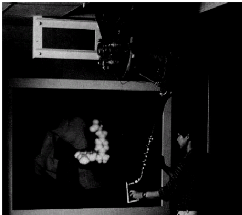
Figure 1: The Docker application simulates the forces between a drug and its receptor site in a protein as the user guides it to the minimum-energy configuration.
