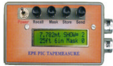
Front panel display window and function buttons. A recalled measurement is shown.
