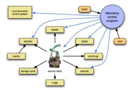
Figure 3: The architecture of the automation system for the laboratory in [9]. The control of the motion sequences of the mobile robot and the path planning between the different biotechnological devices is implemented with the Roblet®-Framework.
