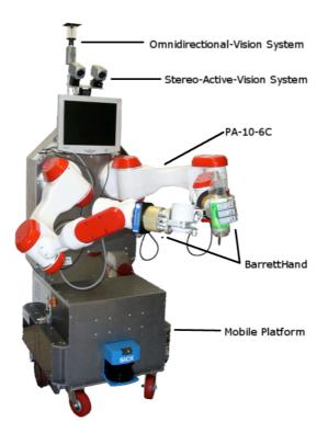
Figure 1: The multimodal service robot TASER of the TAMS Institute at the University of Hamburg.
