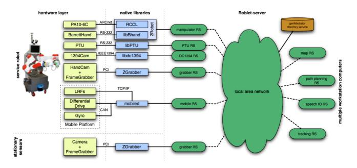
Figure 5: The software architecture of the presented robotic system: Roblet®-servers (RS) are used to provide a hardware abstraction layer. Generalization is realized by this hardware abstraction. Distributed applications are independent of the particular hardware of the robot system. Some Roblet®-servers and connections are left out for clarity.
