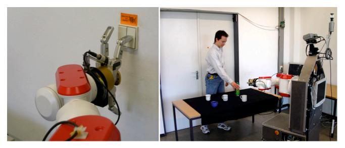
Figure 7: Left: TASER is operating a double-switch. Right: TASER is instructed to grasp a cup by speech and gesture.
