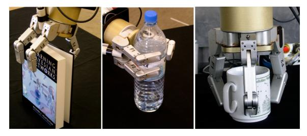
Figure 4: The images show different grasps that can be accomplished by the BarrettHand. These grasp are available as high-level functions through a library encapsulating the control software of the BarrettHand.
