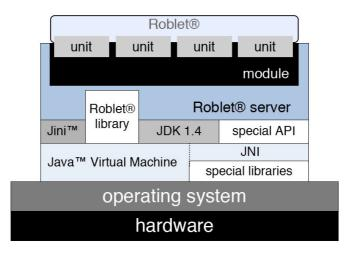
Figure 6: The chart shows the structure of a Roblet®-server and how it hides the hardware from a Roblet®.
