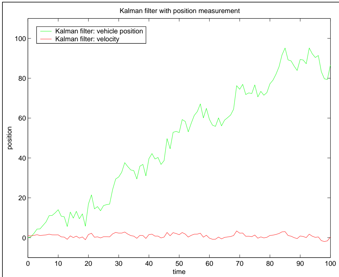
Figure 3.3: MonoRob - Result of the Kalman filter with measurement of the position
