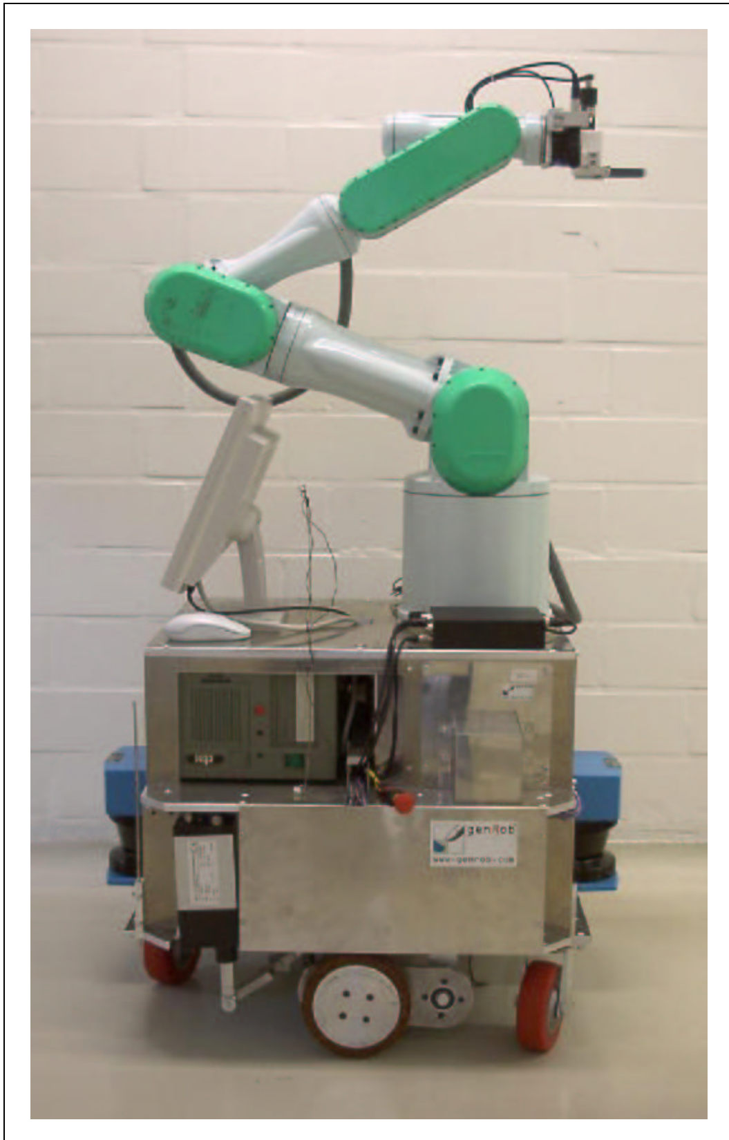
Figure 1.4: The figure shows a photograph of the mobile platform GenBase II with a PA-10 manipulator arm mounted on top.
