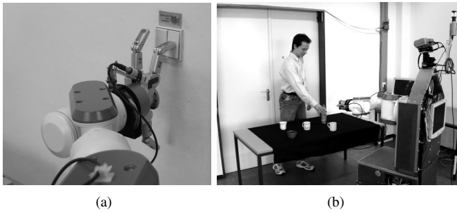
Fig. 5. Left: TASER is operating a double-switch. Right: TASER is instructed to grasp a cup by speech and gesture.
